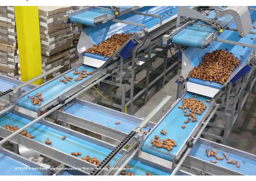
Combining our deep knowledge of the fresh produce industry with rigorous engineering and quality manufacturing to build the best 4-belt even flow accumulator available: the XTR100.
