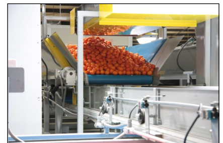
Can Deliver Product to Multiple Distribution Conveyors, with Telescoping Unit Shown Above
